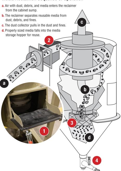
The media reclaimer maintains an effective media working mix while simultaneously removing dust and debris from the blast system. This process ensures consistent blasting results and peak blast system performance.
